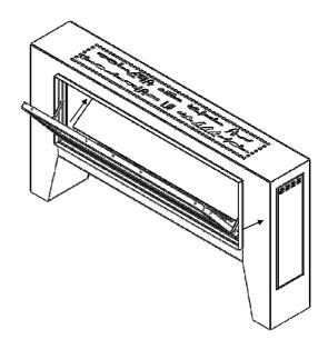
Let the black mirror slide slowly, without dropping it, to fit into the lower mounting bracket. (E)
