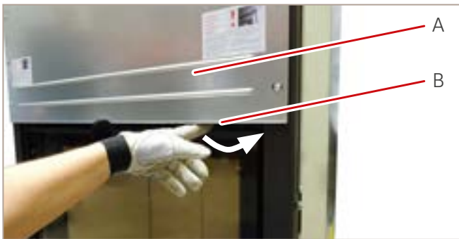
Fig. 27: Locking tongue closed
