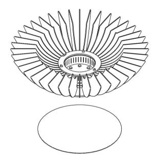
Install the glass with the help of the grooving in order to be fix.
