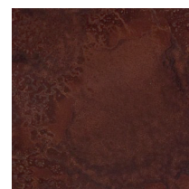
Rusted corten steel
