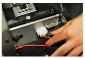
Figure 7—System battery connector location.
