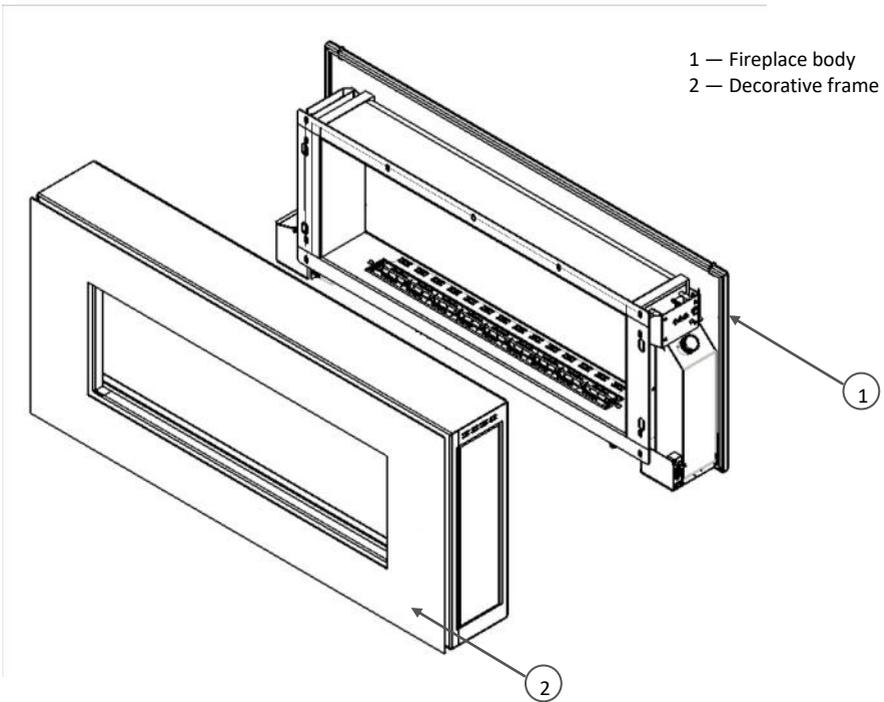
Place the fireplace in the desired location and mark the four holes required on the wall to install it, using the supplied template .
