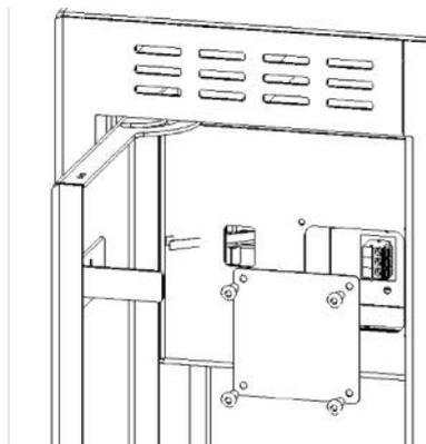
To connect the electric wires slide easy connection of the burner plug, insert the electric wire and release the connection (Figure 3).
