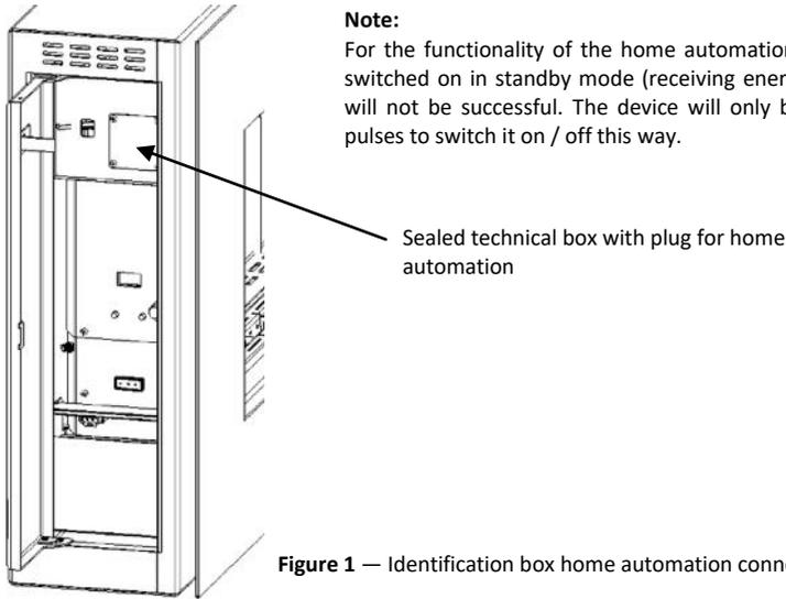
To connect to the home automation system, unscrew the four screws from the technical box and remove the existing protective cover (Figure 2).
