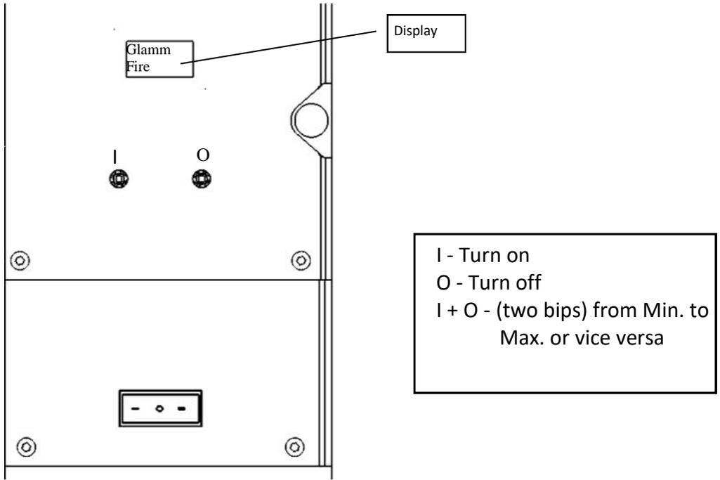
Before connecting the Crea7ionEVO PLUS system, you should select the power supply source—battery or electric current. To do it, select desired option using the **ON/OFF/ON** button, as shown in **Figure 4**.
