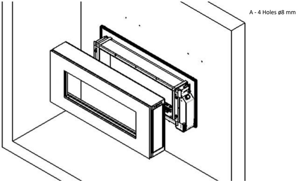
To complete the installation of your fireplace fit the decorative frame and tighten the nuts provided.
