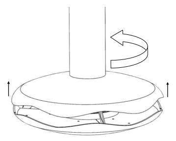
Rotate the dome up, in order to place and filling-in the Burner.
