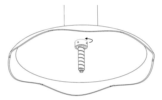
Finally, screw the element (F) to the element (D), using the provided ring and bolt.
