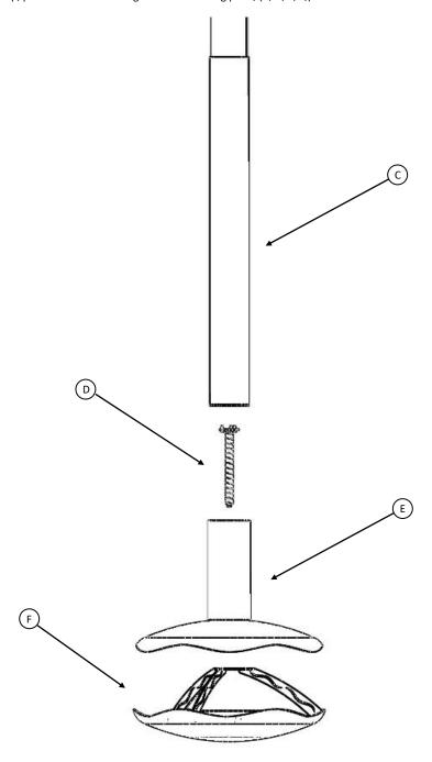
Start the assembly with the fixation of the element (D) to the structure (C), using the holes found at the bottom of the structure (C), with the provided screws.
