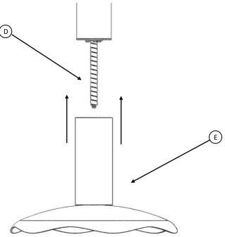
Bolt in the element (E) coupling to the rod thread (D).
