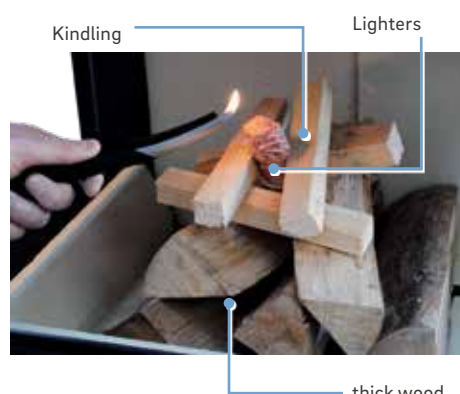
Fig.: 9 Example of igniting process, use log quantity in accordance with the specification „23 Scheitholztabelle“ on Page 48.
