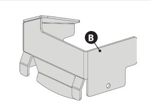
When cleaning and removing the burn pot, remove the flame guard (B) by lifting it. Perform the same operation in reverse order to re-assemble. After having re-positioned, always make sure:
