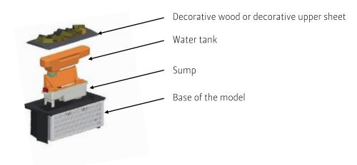
NOTE: The Kit Glamm 3D Plus with water mains connection does not have the tank.
