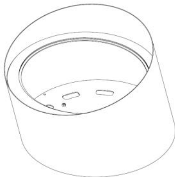
Figure 8- Base of the fireplace
