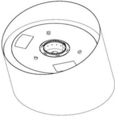
Figure 13 — Burner placed inside Contour
