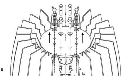
3. Then, remove the vanes from the central shaft (C).
