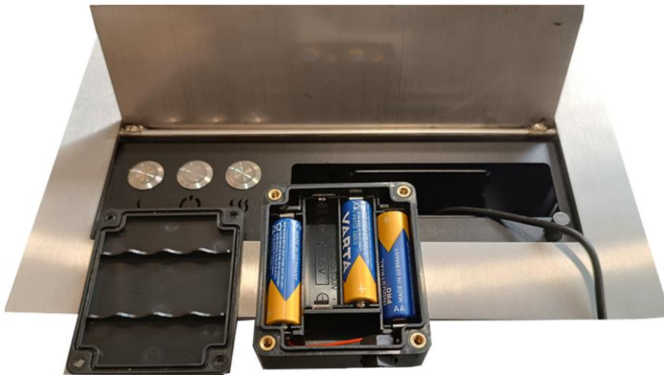
Fig. 11 – Putting back the battery box
