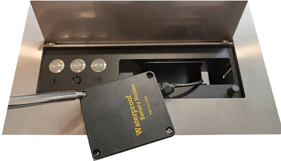
Fig. 10 – Replacing the batteries in the container
