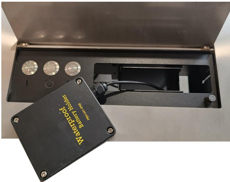
Fig. 9 – Removing of the battery container
