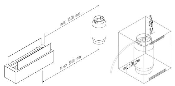
Fig. 5 – Gas cylinder distance and housing for gas cylinder
