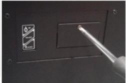
Fig. 11 – Putting back the battery box
