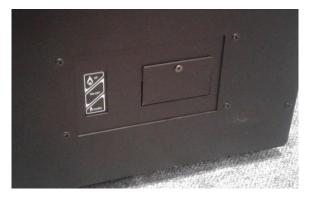
Fig. 8 – Receiver batteries containers
