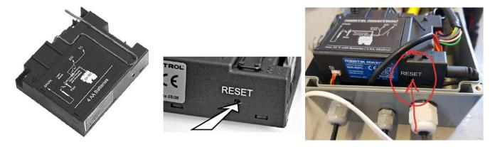
Fig. 7 - Receiver "RESET" button
