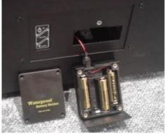
Fig. 10 – Replacing the batteries in the container
