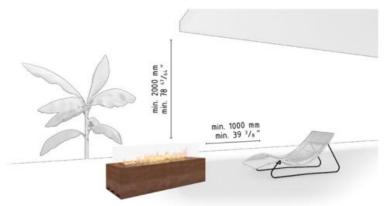
Fig. 1: Minimum distance to flammable materials
