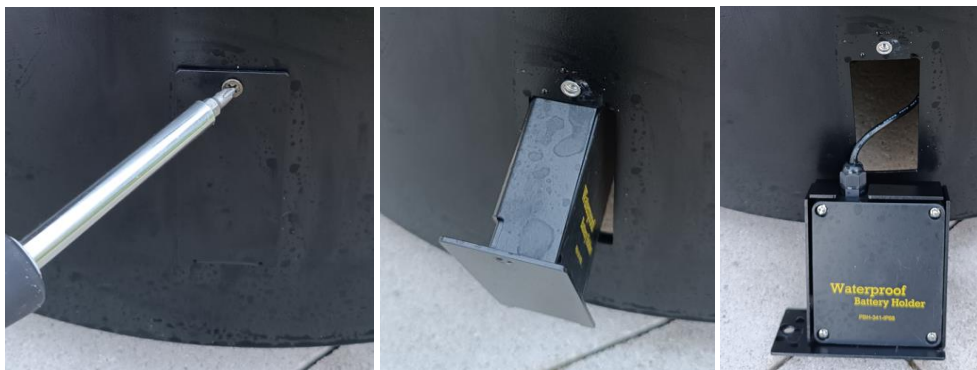
Fig. 8: Removing of the battery container
